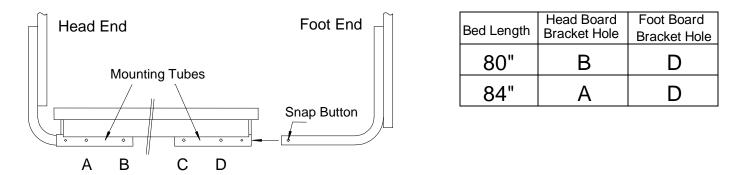
Normally the cap nuts are installed in the head and foot boards at the factory. If they are not installed at the factory, insert the cap nuts provided in the hardware bag into the pre-drilled holes in the head and foot boards using a rubber mallet. If laminated on one side only, install the nuts on the laminated side of the board. Attach head and foot boards to the front face of the vertical bracket using the provided screws. Tighten all hardware.
