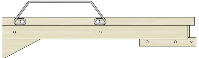
3. Place washer behind deck hole. Align all three holes and insert bolt. Secure with nut, tightening with a  $\frac{1}{2}$ " wrench and a  $\frac{3}{16}$ " Allen wrench. Repeat for other end of Side Mattress Retainer.
