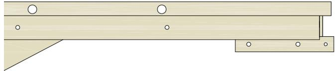
2. Place Side Mattress Retainer against the deck, lining up the outer holes on the Side Mattress Retainer with the deck holes.
