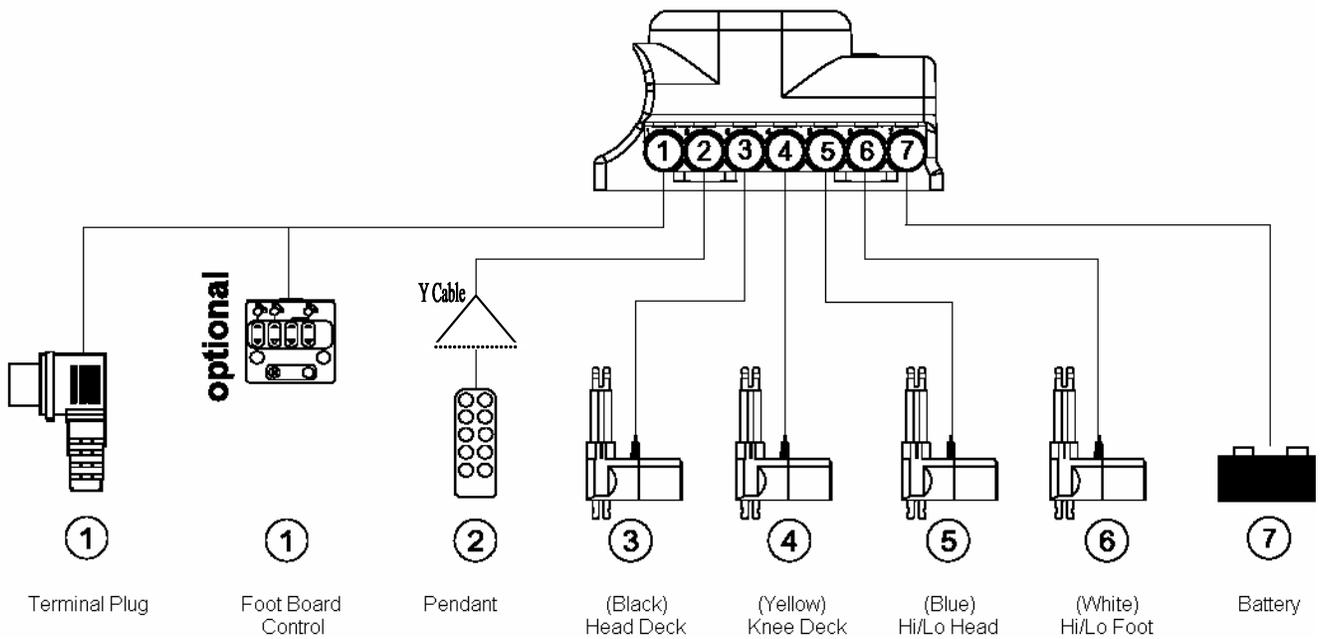
**Note:** The Foot Board Port of the MCL Control Box must have **either** a foot board control extension cable with a terminator plug or a foot board control cable **or** a terminator plug connected directly to the control box for any of the bed functions to operate. All beds are shipped from the factory with a terminating plug connected to the foot board port of the MCL Control Box or at the end of an extension cable plugged into the MCL Control Box.
