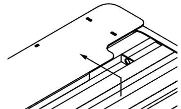
3. Secure the deck extension(s) by replacing the Phillips head screws that hold down the deck extension.
