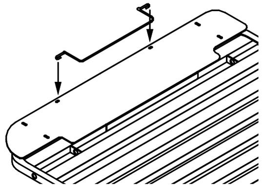
3. With the leg of each side of the End Mattress Retainer positioned in the  $\frac{1}{4}$ " holes, rotate the Retainer outward.
