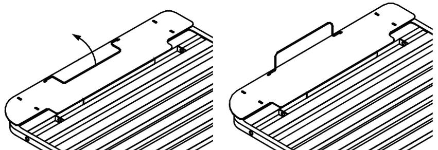
4. Place the mattress on the rib-deck sleep surface. Check that all edges of the mattress are within the Retainers. A slightly compressed fit is desired. Ensure that the Retainers hold the mattress securely to prevent mattress slippage during head and foot deck articulation.
